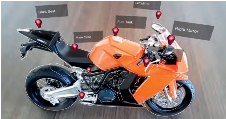
Figure 12: Example of AI object tracking. A deep neural network is used to match the virtual model of a motorcycle (white lines), including the tags, on a real physical object of a motorcycle ( https://www.ptc.com/en/products/vuforia ).
