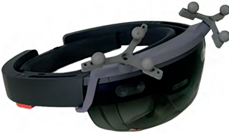
Figure 1: Microsoft HoloLens with frame. Using the reflective markers on the frame, the position of the HoloLens was tracked by the optical tracker.
