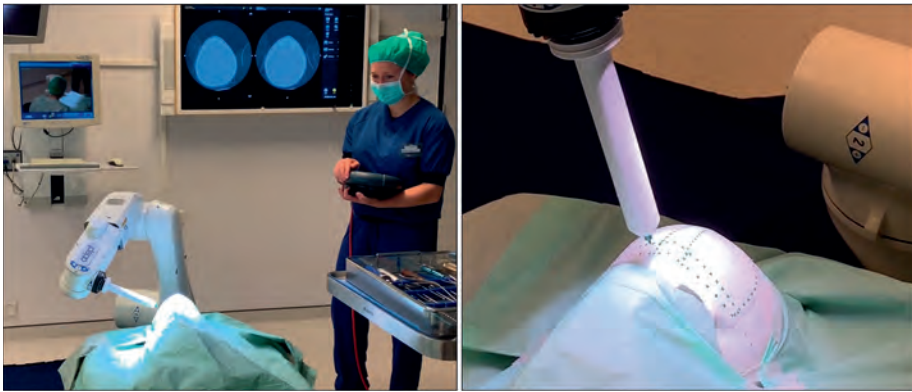
Figure 14: Robotic assisted demarcation of virtually planned osteotomy lines on a craniostylosis patient. Experimental set up in collaboration with Twente University.
